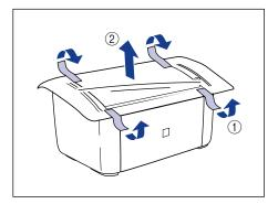
2 Remove the following pieces of tape that are attached to the printer (6 locations).
