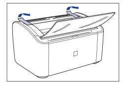
5 Open the multi-purpose tray. Grasp the groove in the center of the printer to open the multi-purpose tray.
