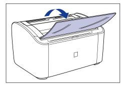
4 Remove the following pieces of tape that are attached to the printer (2 locations).
